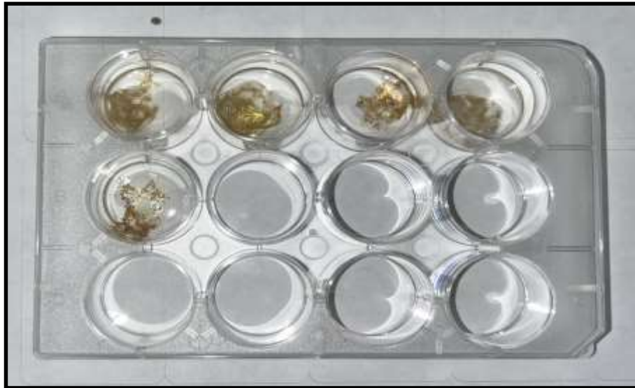
FIG 3: Control sample and study sample in saline solution to determine swelling and degradation rate.
