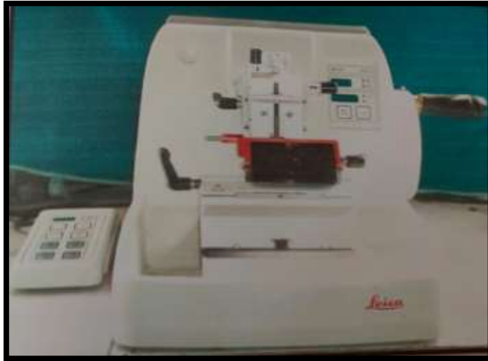
Figure 2: Semi – automatic microtome for preparation of paraffin sections
