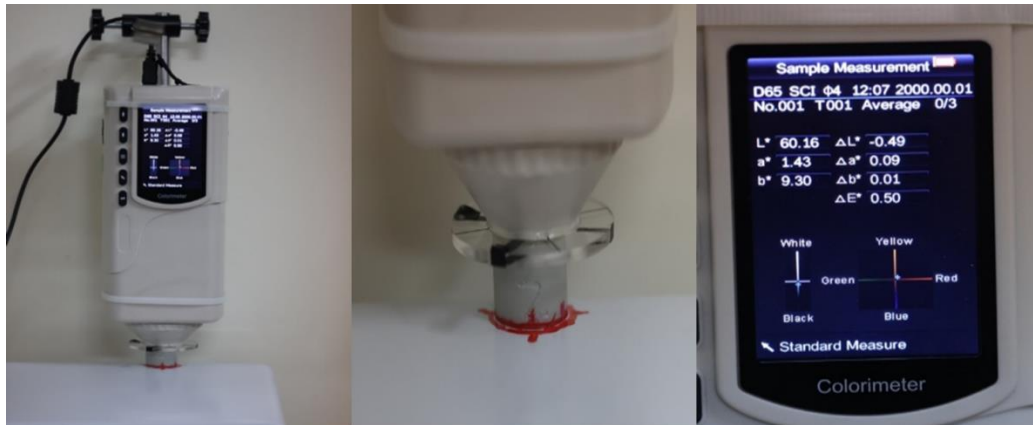
Figure 4. The colorimeter, sample standardizing, and final result display. a. NR110 colorimeter device that has been fixed to the clamp. b. the standardized sample position. c. The digital screen that displayed the Final results.
