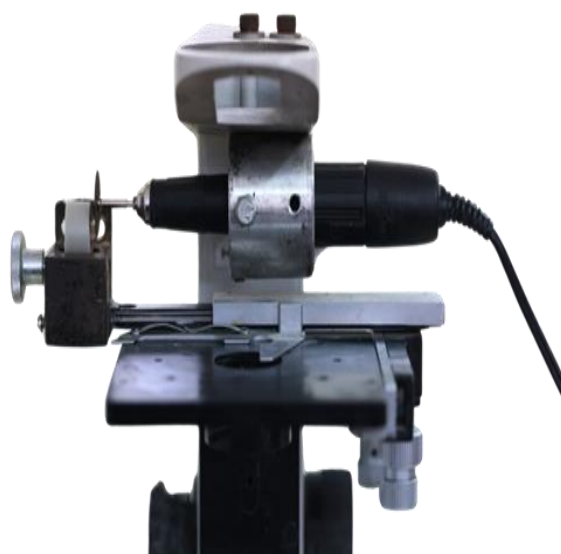
Figure 1. A standard position handpiece affixed to a locally modified adjusted horizontally graduated microscope base.
